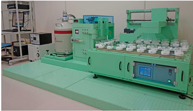
Standard Electrode Coaxial Ge Detectors (with auto-sampler ) 50 samples on the table
