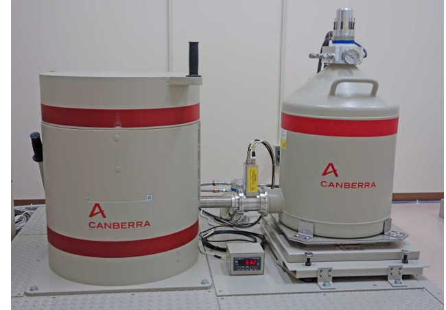
Ultra low background Ge detector (well type 150mL)
